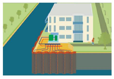
scale renovation projects of the canals and quay walls in the city centers. In Amsterdam alone approximately 200 km of quay wall is in dire need of renovation. By outfitting these steel sheet pile as Energy Sheet piles these structures can attain an additional secondary function as an infinite source of energy.
